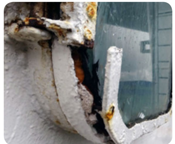
The steel integrity of the MISTRAL's hull structure can't be much better than this less-than-watertight window photographed by Paris MOU inspectors in 2017.
