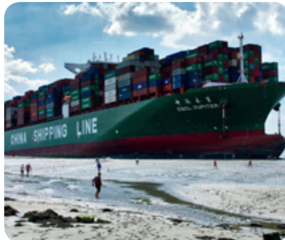
Ultra Large Container Ship M/V JUPITER grounded on Scheldt River bank shortly after departing Antwerp
